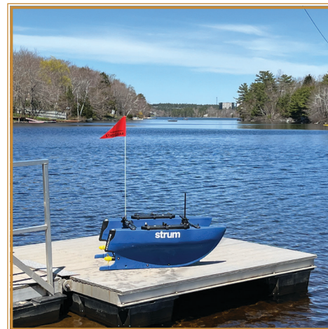
Uncrewed surface vessel used to remotely survey the seafloor and lake beds
